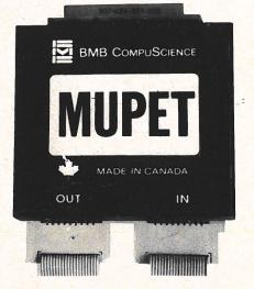
The multiuser disk system functions identically with any Commodore PET\*/CBM and disk combination. In other words the MUPET operates under the same set of commands as those provided in both the CBM User Manual (p/n 320856-3) and the Disk Manual (p/n 320830-4) operating manuals. External work stations function completely independently of each other. The MUPET will operate with software in BASIC, PASCAL, or ASSEMBLY languages, as well as supporting disk files.
