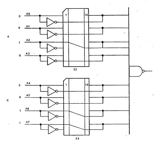
Positions E4 and E5 contain the user-jumpered 16-pin address selection sockets. These jumpers allow the PIC-8 board to respond to any 1 of the 256 possible I/O port addresses.
