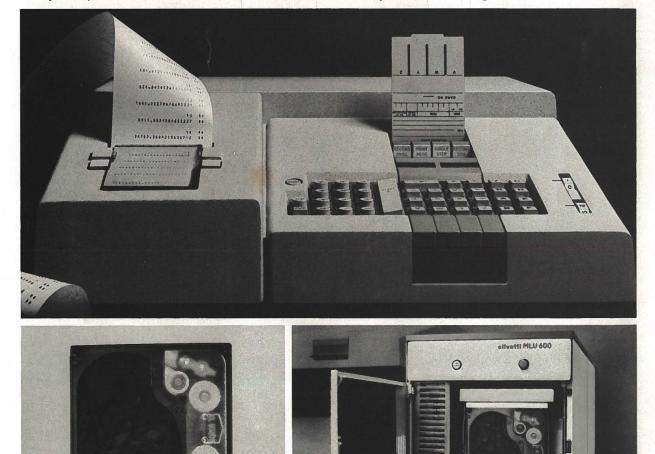
**Capacity**—to handle 400 sides without re-entry. The MLU 600, an information storage unit utilizing advancements in magnetic tape technology, can store and retrieve data under program control without slowing down the operator. Tapes can be removed intact, so that rush, small jobs can be run without disturbing the progress of larger ones.
