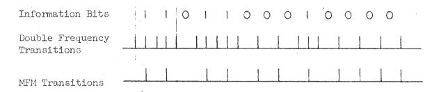
As is illustrated by the timing diagram, the highest and lowest frequency involved in MFM is 1/2 the corresponding frequency for double frequency code at the same data rate. Therefore twice the data rate is available for the same transition rate.
