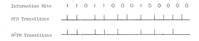
As is illustrated by the timing diagram, the highest frequency in  $M^2FM$  is the same as in MFM. However, the lowest frequency in  $M^2FM$  is 4/5 the lowest frequency in MFM. Also note that clock bits in  $M^2FM$  are not as close to other transitions as in MFM.
