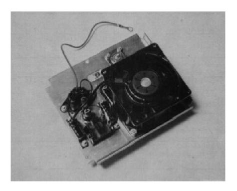
Figure 2-1. Sol-20 fan closure plate assembly. (Top of plate in foreground.)
