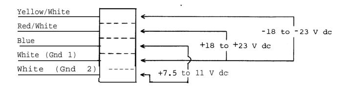
Figure 2-7. Sol-20 power connector and voltage measurements.
