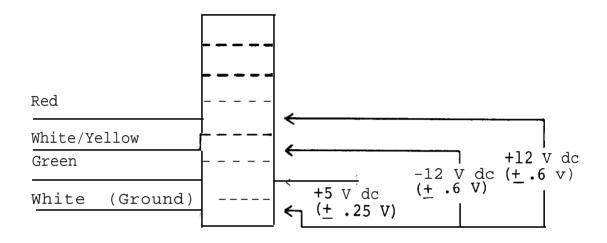
Figure 2-6. Sol-PC power connector and voltage measurements.
