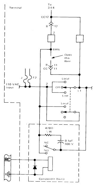
TTY Terminal Schematic Incorporating Automatic Reader Control
