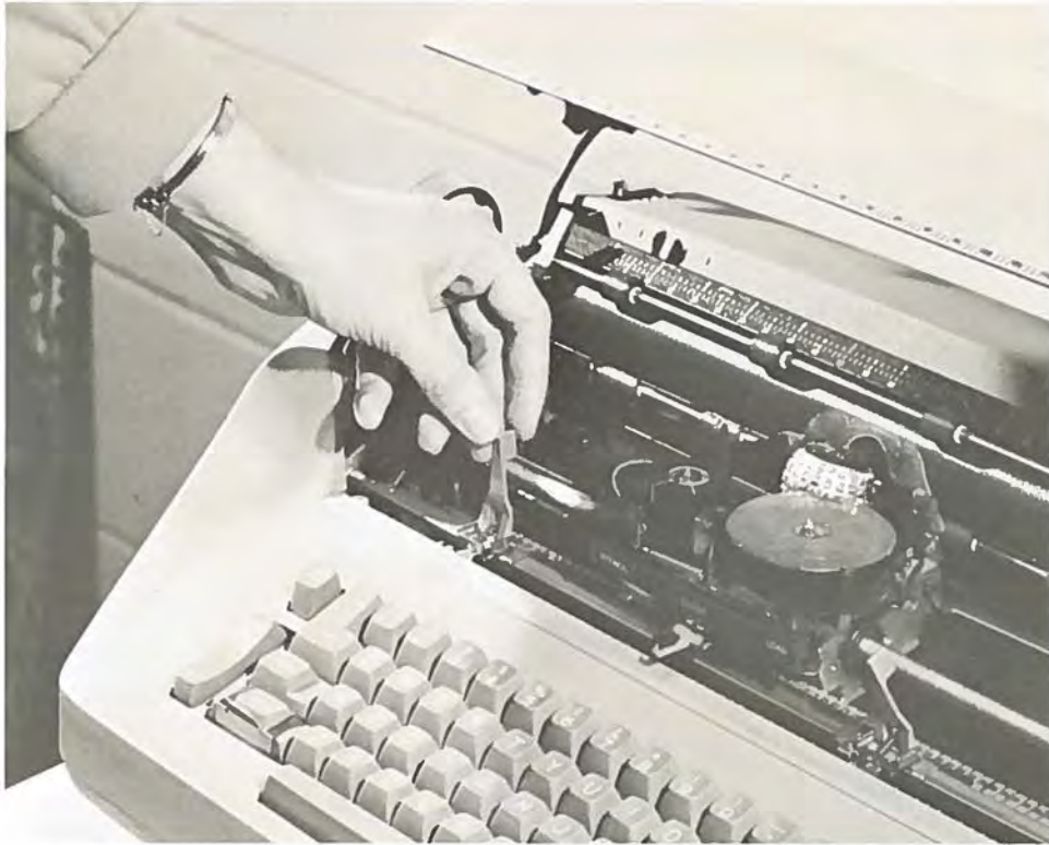
Figure 3-2. Lift the cover of the Selectric, then lift both margin stops.
