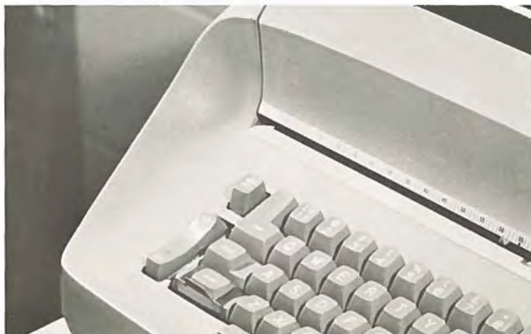
Figure 3-1. Place the clip provided with Printing Robot on the Selectric®SHIFT key.
