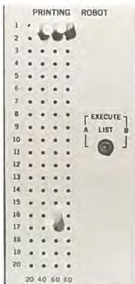
Figure 2-3. Tabulation controller with pins set for subscription list example.
