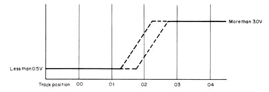
Adjust so that the level of the sensor output changes between track 01 (Low level) and track 03 (High level)
