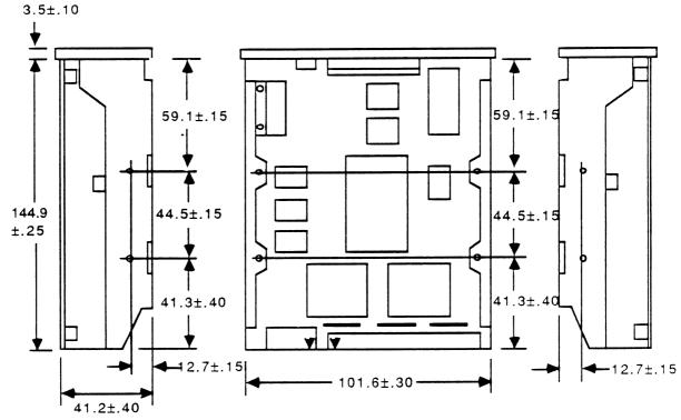
DIMENSIONS ARE IN MILLIMETERS; SCREW SIZE IS 6-32
