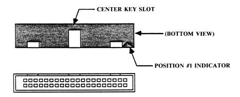
FIGURE 2 — AT-BUS INTERFACE CONNECTOR (J2)
