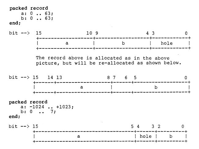
In the last example above, the signed subrange field was moved up to the left hand end of the word and sign extended for faster access.
