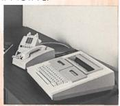
vides serial data I/O compatible with EIA Standard Interface specification RS232/C, as well as standard protocols for ASCII, IBM Correspondence Code and Tektronix 4013 Graphics.
