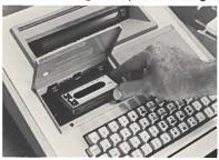
storage drives that expand the memory capacity by more than 200,000 words. Also included is a resident operating system which includes: a Virtual Operating System, Omniport Input/ Output Interface, a complete APL interpreter, and a battery-operated Power Fail Protection System
