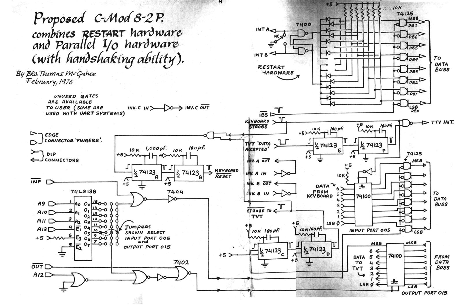
Note: with the exception of the capacitor values used, each pair of 74123 one-shot functions is wired identically.
